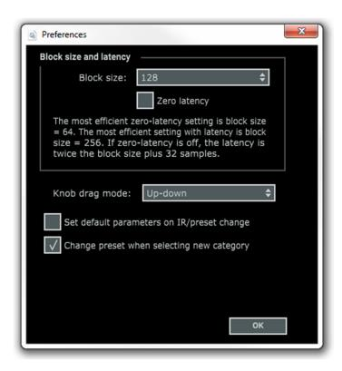
The top section sets the internal block size and latency of the convolution engine. The default setting is a compromise between fast performance (low CPU usage) and low latency. Clicking the "Zero latency" button enables zero latency mode, which means the plug-in does not delay the output at all. Zero latency consumes more CPU.
