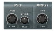
Predelay is a standard reverb control that simply delays the wet response.
