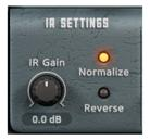
Normalize will automatically apply gain so that the wet reverb sounds equally loud as the dry sound. If Normalize is off, you can dial in the gain yourself using the IR Gain control. The IR Gain control has no effect if Normalize is enabled. The Reverse control time-reverses the IR.
