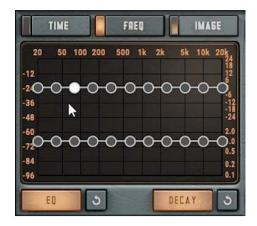
Clicking the EQ button enables EQ editing and a set of 11 control handles appear at the top of the graph. The handles let you draw an EQ curve, with a large range of -24 dB to +24 dB. Clicking the reset (circular arrow) button resets the EQ to no modification, i.e., 0 dB at all frequencies.
