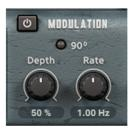
The 90 degree option modulates the stereo channels in quadrature (sin/cos) phase. The Depth sets the amount of modulation, and the Rate sets the rate of modulation.
